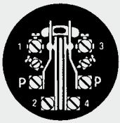
Contact assembly for clock or anti-clockwise rotation
